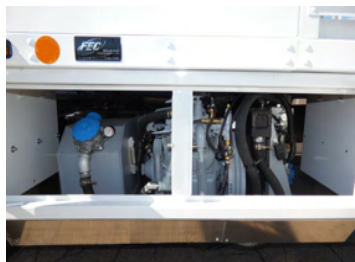
Air compressor with PTO/hydraulic drive available under floor or in bed.
