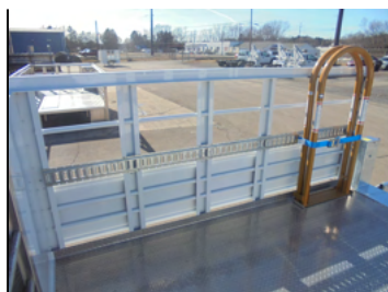
E-track installed on all service bodies for strap application. Tire inflation cage available for safe inflation.
