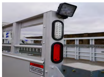
LED tail lights are standard. Optional 3-way and 4-way LED strobes systems available. High power LED work lights can be installed for improved visibility.
