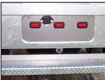
7-pin trailer plug available for testing trailer lights. Optional backup camera for safety while reversing.
