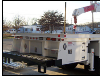
Optional rear step and grab handle for easy access to the bed.
