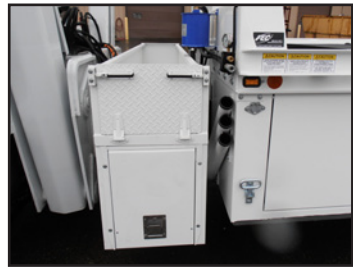
Cross-body block basket with a fold-down side and tool boxes available depending on chassis length and configuration. Sahara air dryer also shown.
