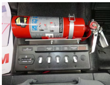
In-cab switch panel used to control auxiliary components. 5-lb. Fire extinguisher secured.
