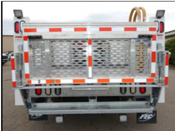
1500 lb. liftgate with heavy duty steel frame and aluminum platform. Self locking two-point spring loaded lock system locks platform closed when stored for travel. Optional self locking tire stacking rack on platform.
