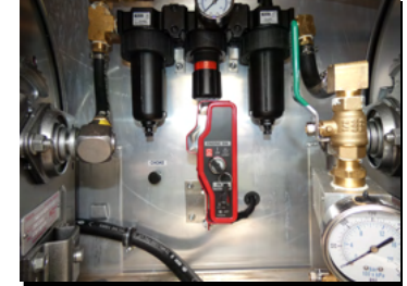
Remote engine controls in right front compartment.
