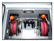
Hose reels available in right front compartment. 1/2" X 50' and 3/8" X 50' heavy duty reels with hose end guard, Optional Air Water Oiler shown.
