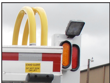
LED tail lights are standard. Optional 3-way and 4-way LED strobe systems available. High power LED work lights can be placed for best visibility.
