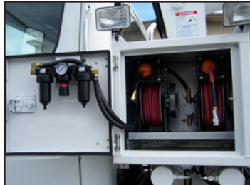
Hose reels commonly placed in slew box on left side. 1/2" X 50' and 3/8" X 50' heavy duty reels with hose end guard,
