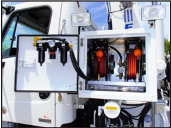
Hose reels commonly placed in slew box on left side. 1/2" X 50' and 3/8" X 50' heavy duty reels with hose end guard, Optional airing station for easy tire inflation is available.
