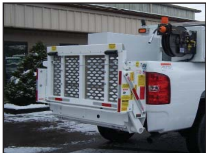
1300 lb. LA56 liftgate with heavy duty steel frame and aluminum diamond tread deck plate. Self locking two-point spring loaded lock system locks platform closed when stored for travel. Powder-coat paint finish.
