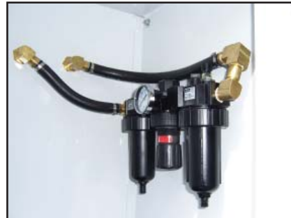
Air, Water, Oiler available in right front compartment.
