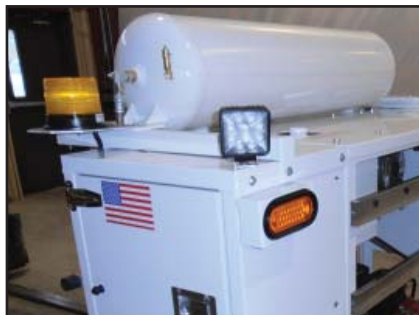
Remote key-fob actuated emergency LED strobe beacon, LED work lights, and rear-facing LED strobe lights with manual override for operator safety.
