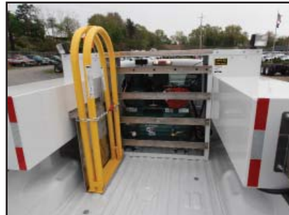
13 hp Honda mounted on 30 gal. air tank 13 hp Honda with 35 gal. overhead air tank 20 hp Kohler with 35 gal. overhead air tank
