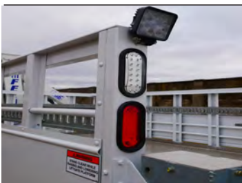
LED tail lights are standard. Optional 3-way and 4-way LED strobes systems available. High power LED work lights can be placed for best visibility.
