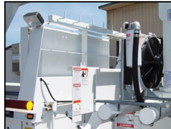
Tire life tank, O-Ring rack, and Heavy-Duty 12V oil cooler for crane and air compressor hydraulics available.
