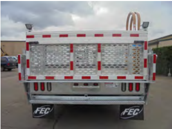
2000 lb. liftgate with heavy duty steel frame and aluminum platform. Self locking two-point spring loaded lock system locks platform closed when stored for travel. Optional self locking tire stacking rack on platform.
