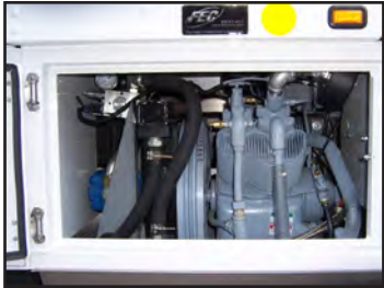
H65DC air compressor with PTO/hydraulic drive available under floor or in bed.
